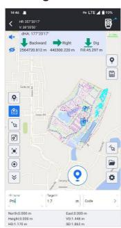
CAD Stakeout allows you to import **CAD basemap** and stakeout it, without input point coordinates one by one.
