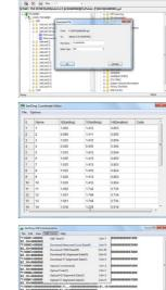
Powerful and convenient data transfer and postprocessing software with concise and clear interface and user-friendly operation. User can download and upload raw data or coordinates in GSI format, edit coordinates and codes, design and edit road data, transfer GSI data to DXF file for processing in CAD, etc.
